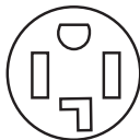
4-wire receptacle (14-30R)
