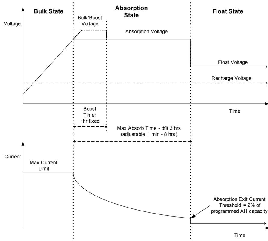
**Figure 1-2** Three-stage Battery Charging Cycle<sup>a</sup>
